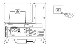
Note: Optional USB devices include the Zultys Bluetooth USB dongle, Wi-Fi USB dongle, ZIP 450M Expansion Module and Electronic Hook Switch Adapter.
