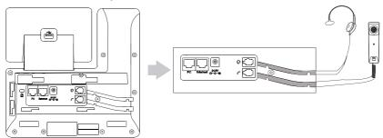
Note: Electronic Hook Switch (EHS) functionality is supported with compatible wireless headsets when used with the optional Zultys Electronic Hook Switch Adapter connected via the USB port.
