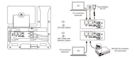
Note: The IP phone should be used with Zultys original power adapter (5V/1.2A) only. The use of a third-party power adapter may cause damage to the phone. If you are connecting a PC to your phone, we recommend that you use the Ethernet cable provided by Zultys.
